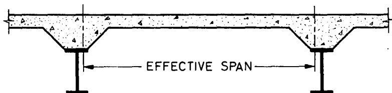
FIG. 1 EFFECTIVE SPAN OF SLAB SUPPORTED ON STEEL PREFABRICATED UNITS
