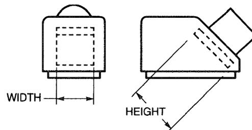
Figure 6.20—Transducer Crystal
