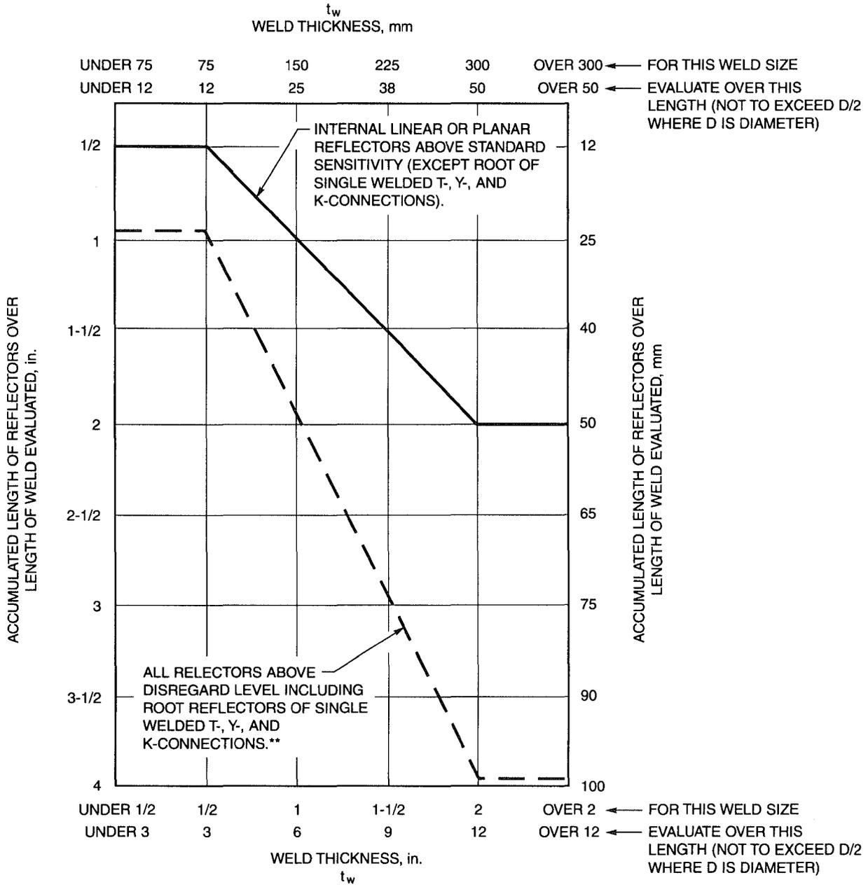
\*\*ROOT AREA DISCONTINUITIES FALLING OUTSIDE THEORETICAL WELD (DIMENSIONS " $t_w$ " OR "L" IN FIGURES 3.8, 3.9 AND 3.10) ARE TO BE DISREGARDED.
