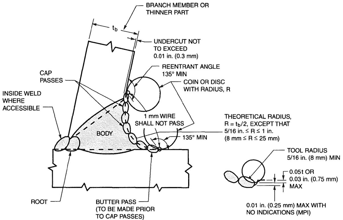
NOTE: MINIMUM REQUIREMENTS FOR OUTSIDE WELD AT TUBULAR CONNECTIONS DESIGNATED TO MEET 2.36.6.6(1).
