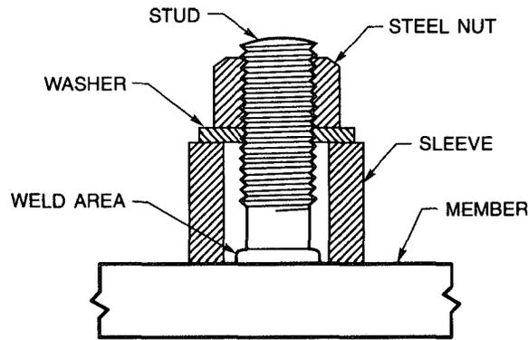
DIMENSIONS OF TEST FIXTURE DETAILS SHOULD BE APPROPRIATE TO THE SIZE OF THE STUD. THE THREADS OF THE STUD SHALL BE CLEAN AND FREE OF LUBRICANT OTHER THAN THE RESIDUE OF CUTTING/COLD FORMING LUBRICANTS IN THE "AS RECEIVED" CONDITION FROM THE MANUFACTURER.
