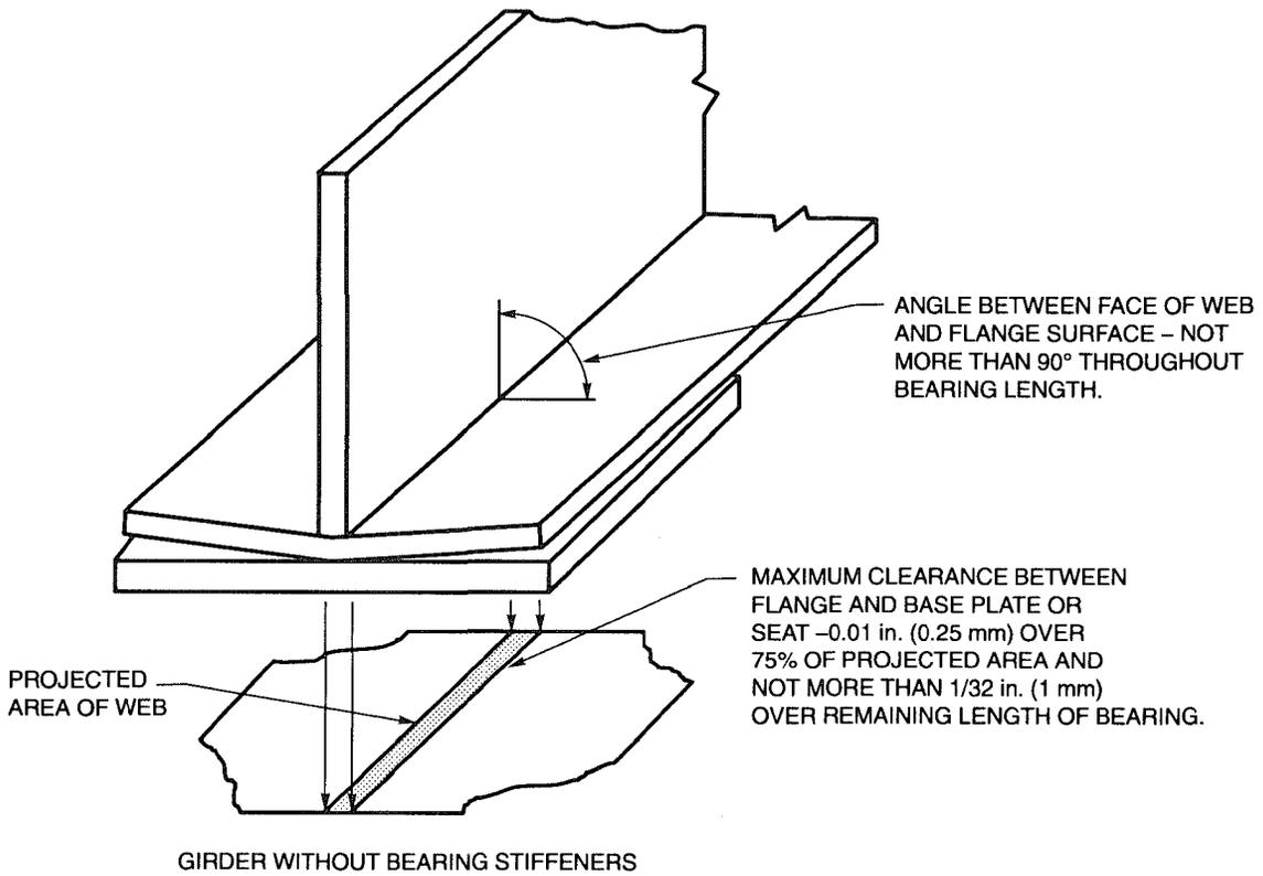
Figure C5.8—Tolerances Bearing Points (see C5.23.10)
