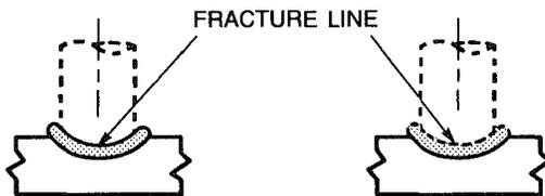
Note: Fracture in weld near stud fillet remains on plate.
