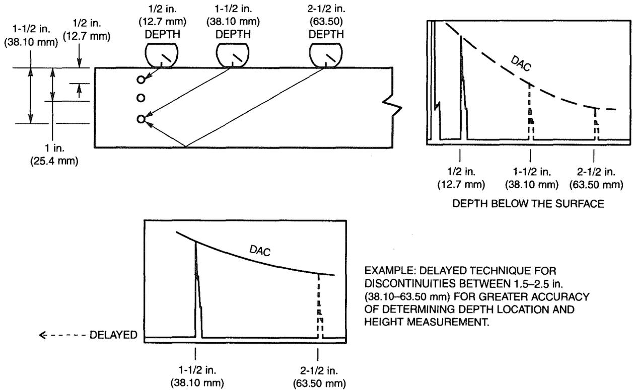
EXAMPLE: DELAYED TECHNIQUE FOR DISCONTINUITIES BETWEEN 1.5–2.5 in. (38.10–63.50 mm) FOR GREATER ACCURACY OF DETERMINING DEPTH LOCATION AND HEIGHT MEASUREMENT.
