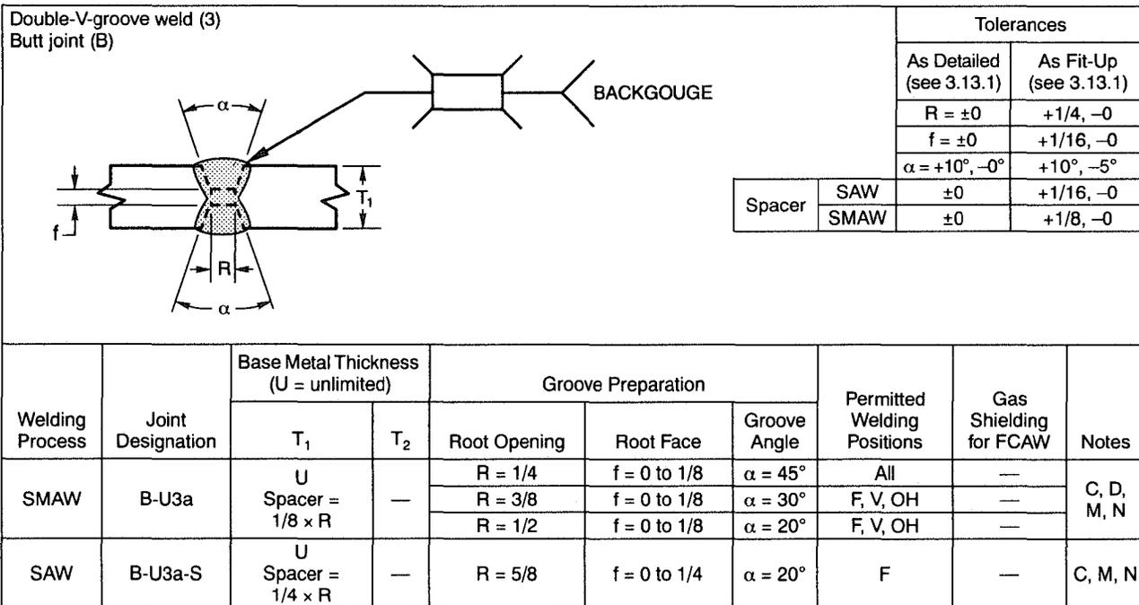
Figure 3.4 (Continued)—Prequalified Complete Joint Penetration (CJP) Groove Welded Joint Details (see 3.13)
