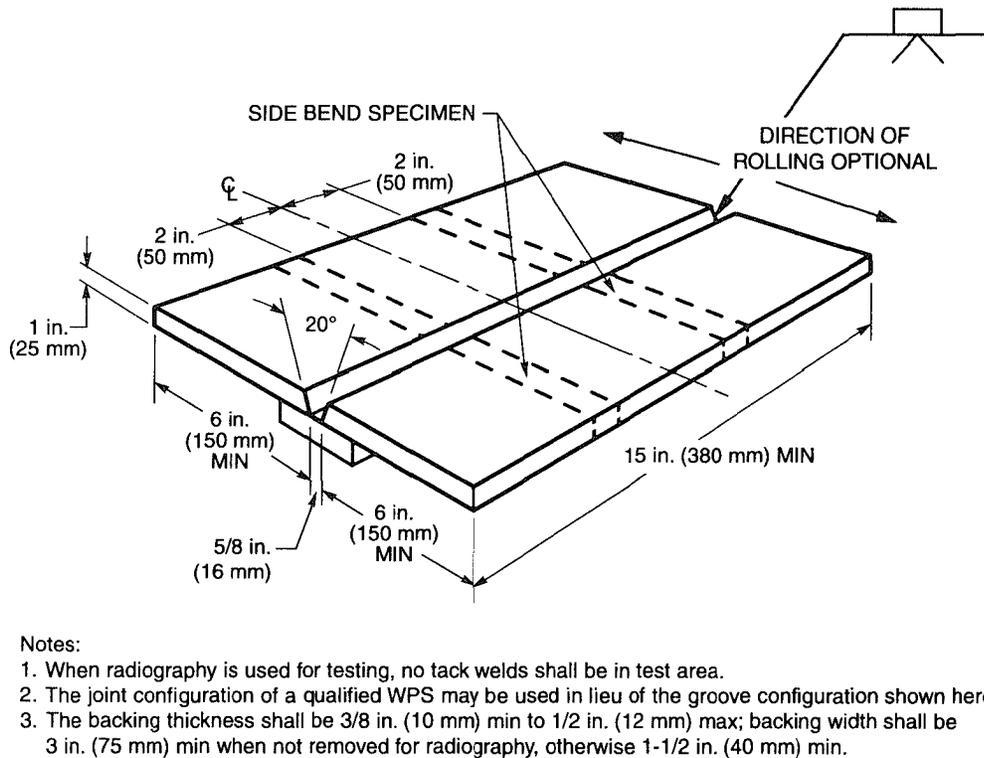
**Figure 4.22—Test Plate for Unlimited Thickness—Welding Operator Qualification (see 4.23.2)**
