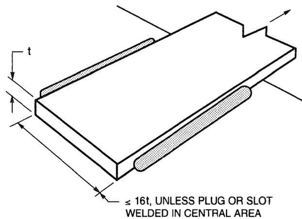
**Figure C2.17—Fillet Welds in End Connections (see C2.32.1)**
