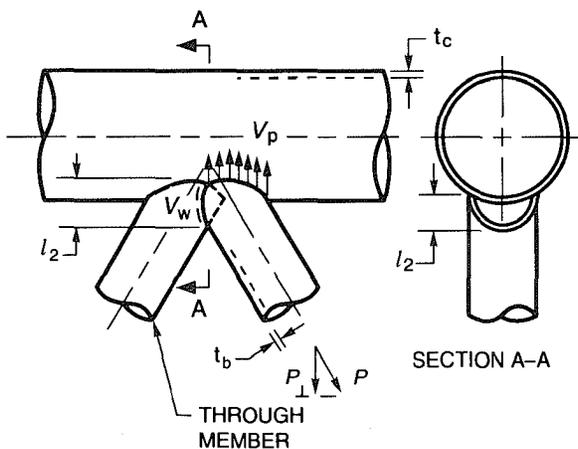
**Figure 2.18—Detail of Overlapping Joint**
