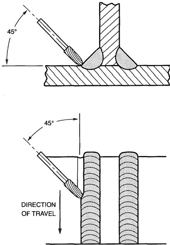
**Figure C8.3—Toe Dressing with Burr Grinder**
