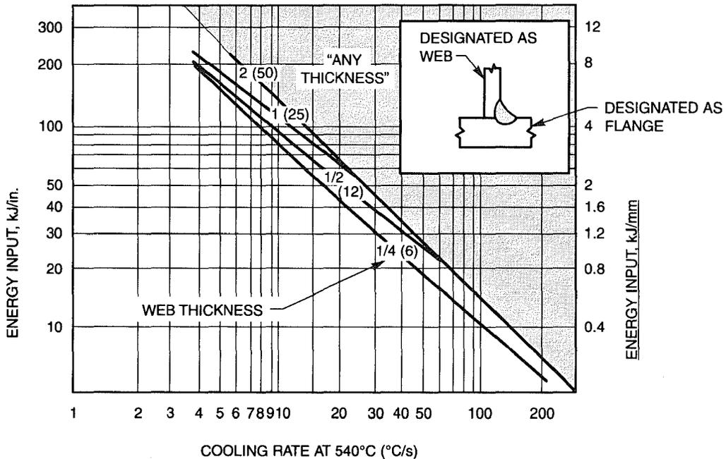
NOTE: ENERGY INPUT DETERMINED FROM CHART DOES NOT IMPLY SUITABILITY FOR PRACTICAL APPLICATIONS. FOR CERTAIN COMBINATION OF THICKNESSES MELTING MAY OCCUR THROUGH THE THICKNESS.
