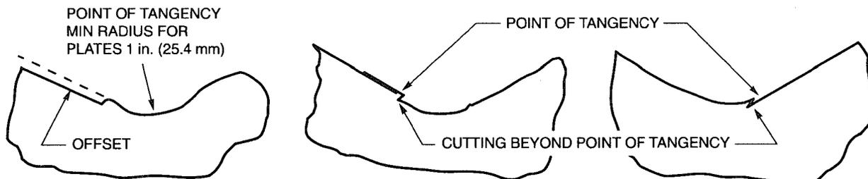
**Figure C5.1—Examples of Unacceptable Reentrant Corners (see C5.16)**
