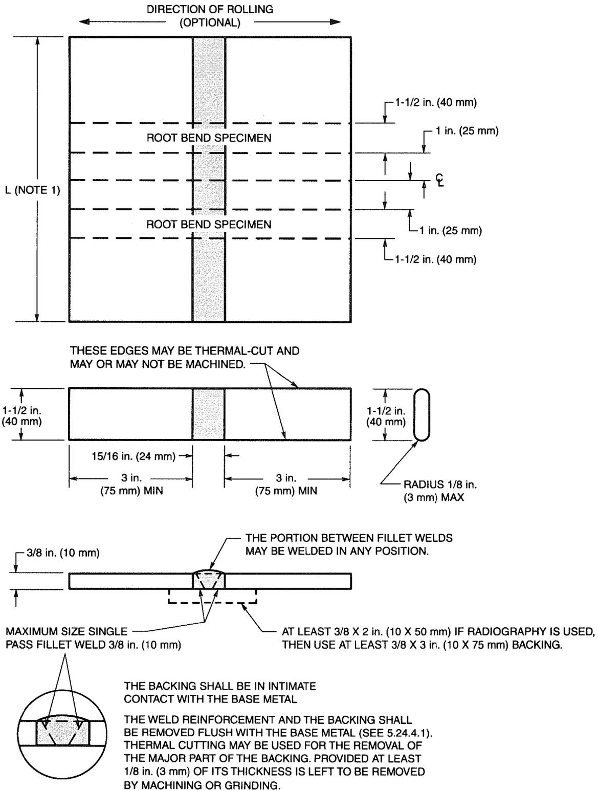
NOTE 1: L = 7 in. (125 mm) MIN (WELDER), L = 15 in. (380 mm) MIN (WELDING OPERATOR).
