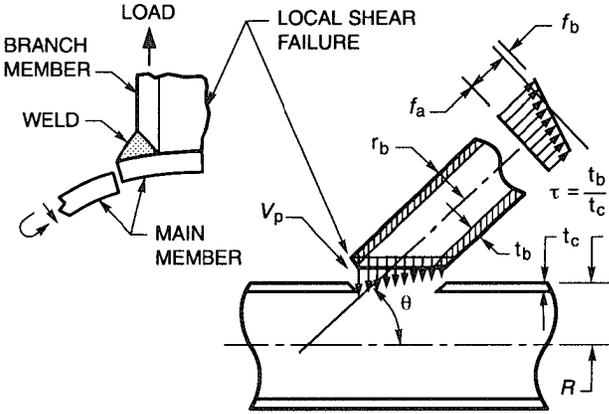
**Figure C2.21—Simplified Concept of Punching Shear (see C2.40.1.1)**
