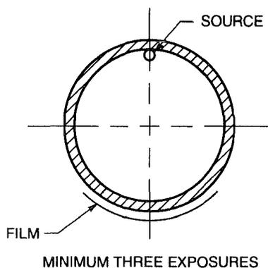
**Figure 6.16—Single-Wall Exposure—
