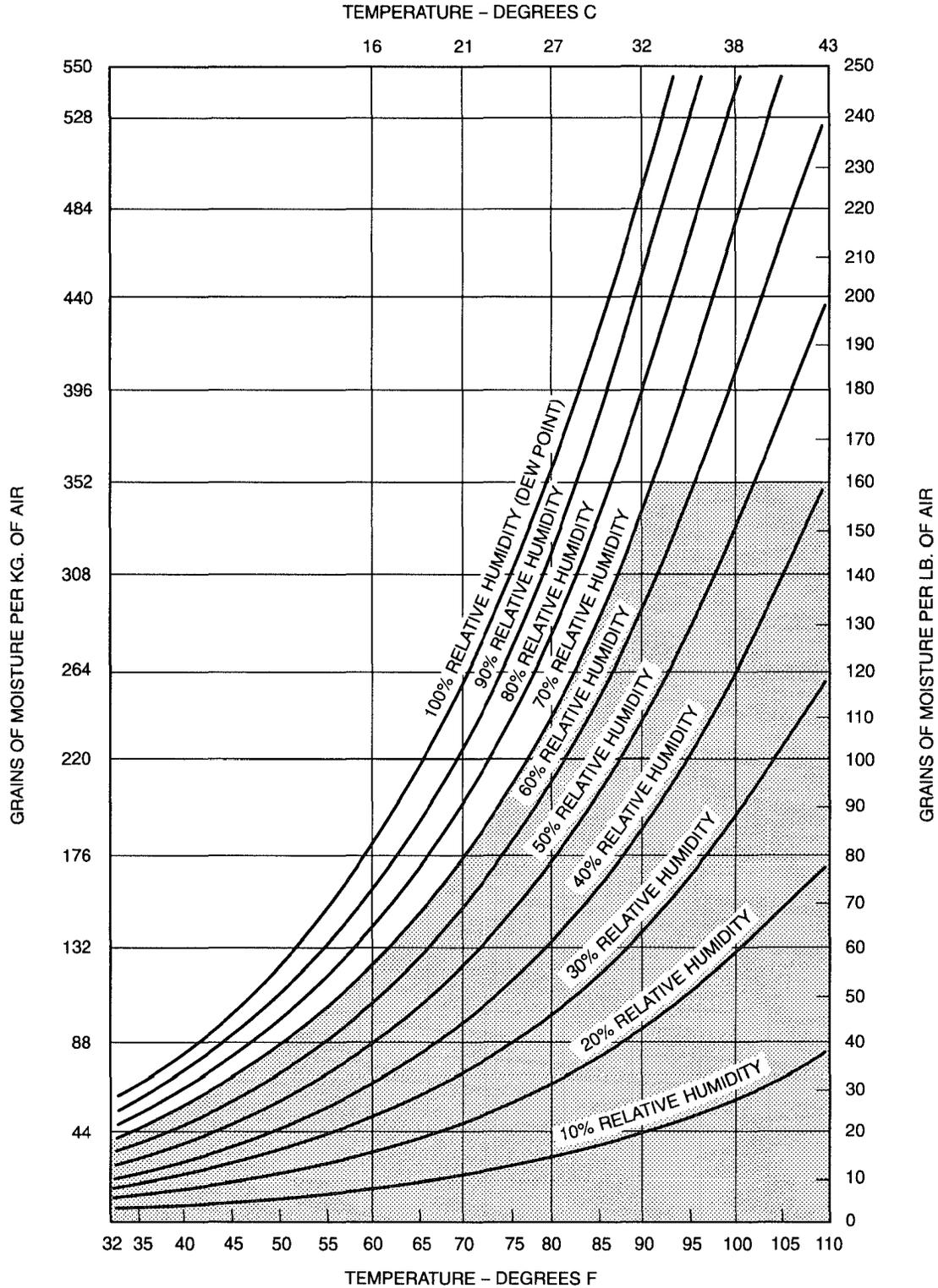
EXAMPLE: AN ELECTRODE TESTED AT 90° F (32° C) AND 70% RELATIVE HUMIDITY (RH) MAY BE USED UNDER THE CONDITIONS SHOWN BY THE SHADED AREAS. USE UNDER CONDITIONS REQUIRES ADDITIONAL TESTING.
