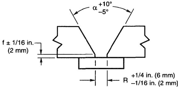
(B) GROOVE WELD WITH BACKING—
