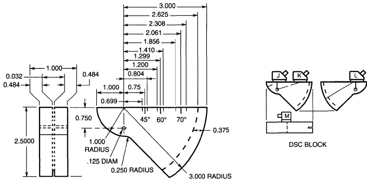
TYPE DSC – DISTANCE AND SENSITIVITY CALIBRATION BLOCK
