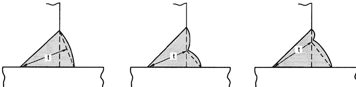
NOTE: THE EFFECTIVE THROAT OF A WELD IS THE MINIMUM DISTANCE FROM THE ROOT OF THE JOINT TO ITS FACE, WITH OR WITHOUT A DEDUCTION OF 1/8 in. (3 mm), LESS ANY CONVEXITY.
