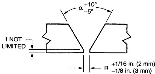
(C) GROOVE WELD WITHOUT BACKING—
