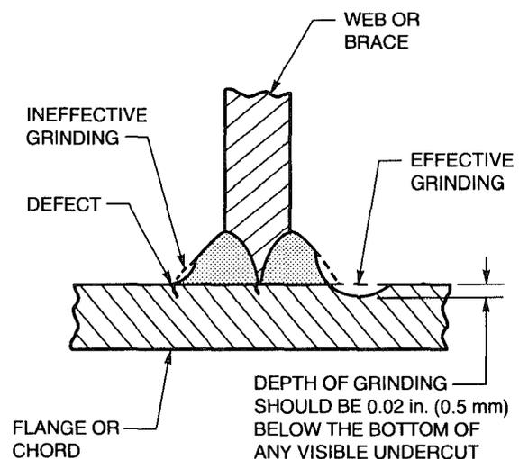
**Figure C8.5—Effective Toe Grinding**
