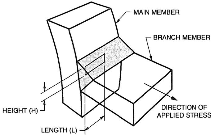
ALIGNED DISCONTINUITIES SEPARATED BY LESS THAN  $(L_1 + L_2)/2$  AND PARALLEL DISCONTINUITIES SEPARATED BY LESS THAN  $(H_1 + H_2)/2$  SHALL BE EVALUATED AS CONTINUOUS.
