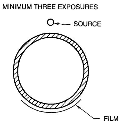
**Figure 6.17—Double-Wall Exposure—
