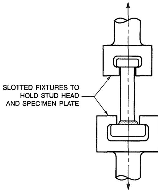
**Figure 7.2—Typical Tension Test Fixture**
