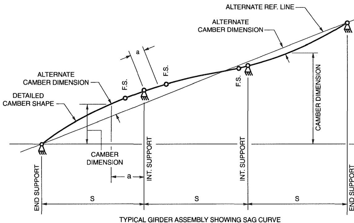
NOTE: PLUS TOLERANCE INDICATES POINT IS ABOVE THE DETAILED CAMBER SHAPE.
