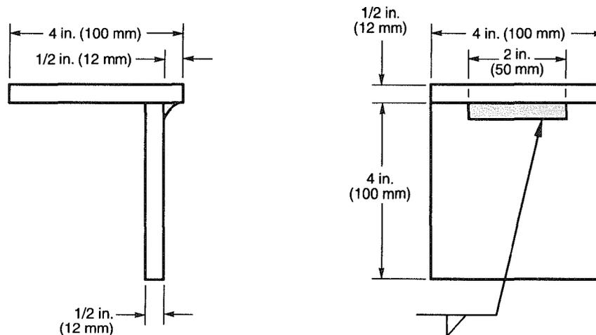
Figure 4.38—Fillet Weld Break Specimen—Tack Welder Qualification (see 4.19.2)
