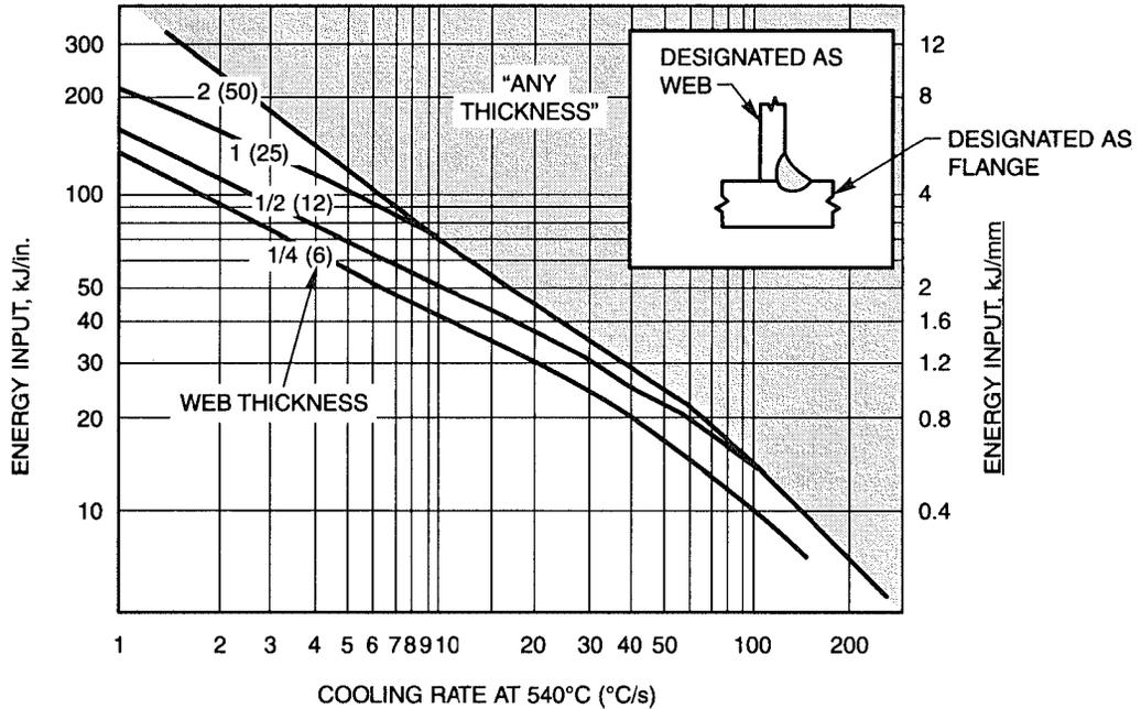
NOTE: ENERGY INPUT DETERMINED FROM CHART DOES NOT IMPLY SUITABILITY FOR PRACTICAL APPLICATIONS. FOR CERTAIN COMBINATION OF THICKNESSES MELTING MAY OCCUR THROUGH THE THICKNESS.
