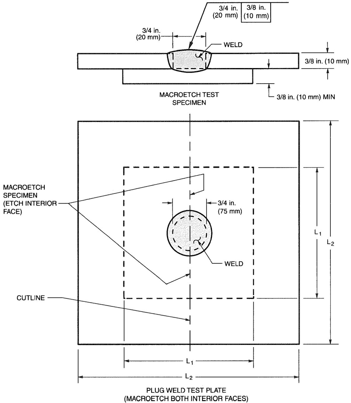
NOTE 1: L<sub>1</sub> = 2 in. (50 mm) MIN (WELDER), 3 in. (75 mm) MIN (WELDING OPERATOR),
