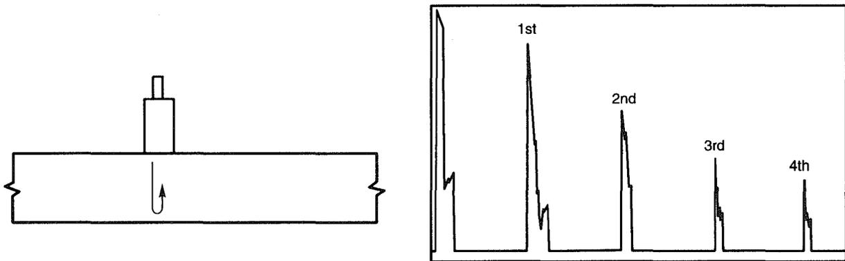
**Figure K-5—Compression Wave Depth (Horizontal Sweep Calibration)
