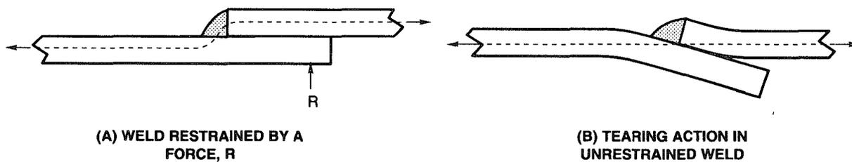
Figure C2.14—Single Fillet Welded Lap Joints (see C2.4.8.1)
