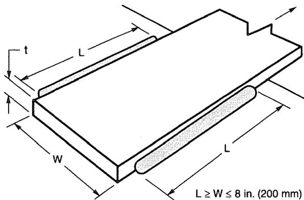
WHEN  $W > 8$  in. (200 mm), TRANSVERSE FILLET WELDS OR INTERMEDIATE PLUG WELDS ARE REQUIRED.
