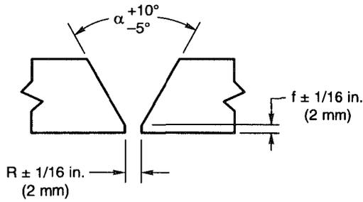
(A) GROOVE WELD WITHOUT BACKING—
