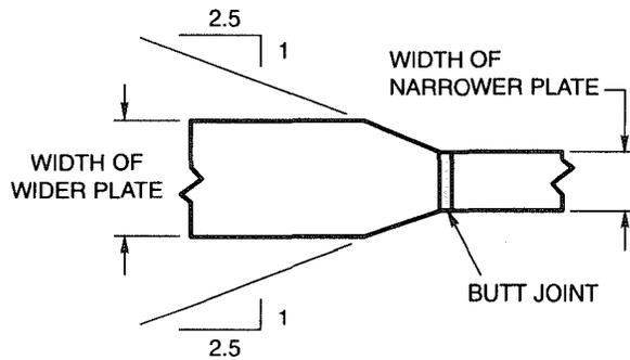
**Figure 2.7—Transition of Widths (Statically Loaded Nontubular) (see 2.20)**
