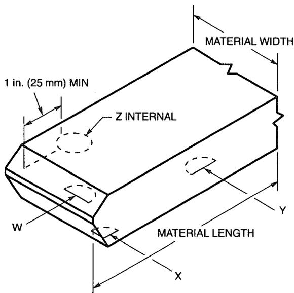
**Figure 5.1—Edge Discontinuities in Cut Material (see 5.15.1.1)**
