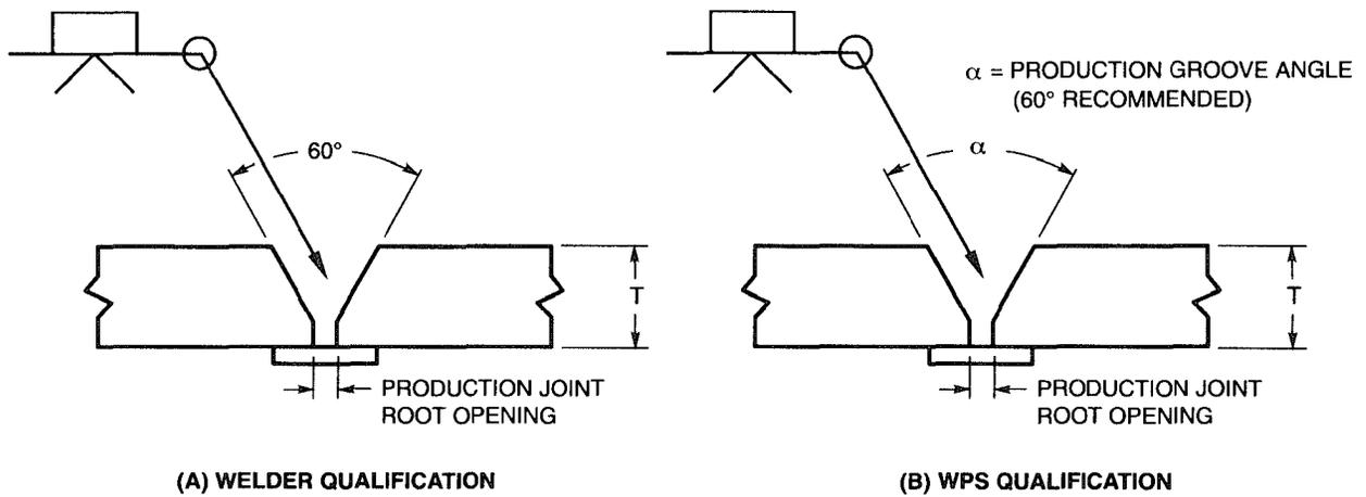
NOTE: T = QUALIFICATION PIPE OR BOX TUBE WALL THICKNESS
