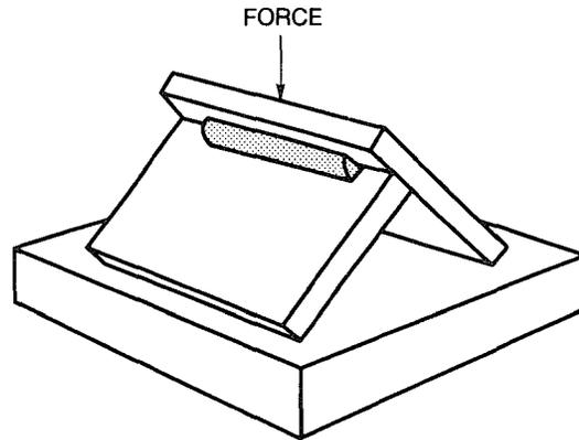
**Figure 4.34—Method of Rupturing Specimen—
