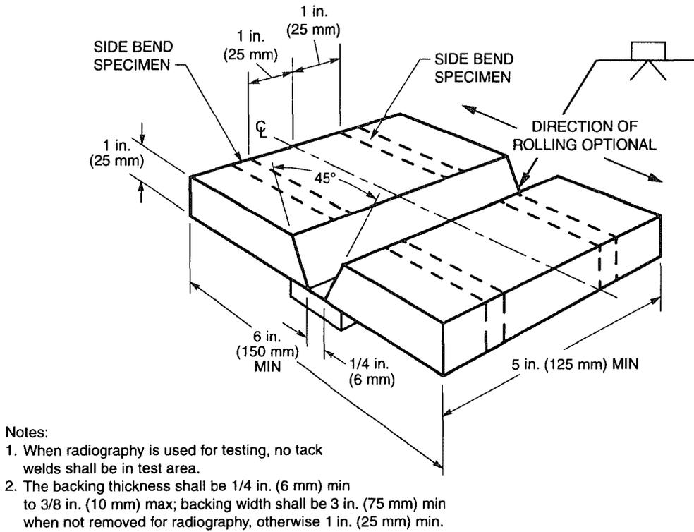
**Figure 4.21—Test Plate for Unlimited Thickness—Welder Qualification (see 4.23.1)**
