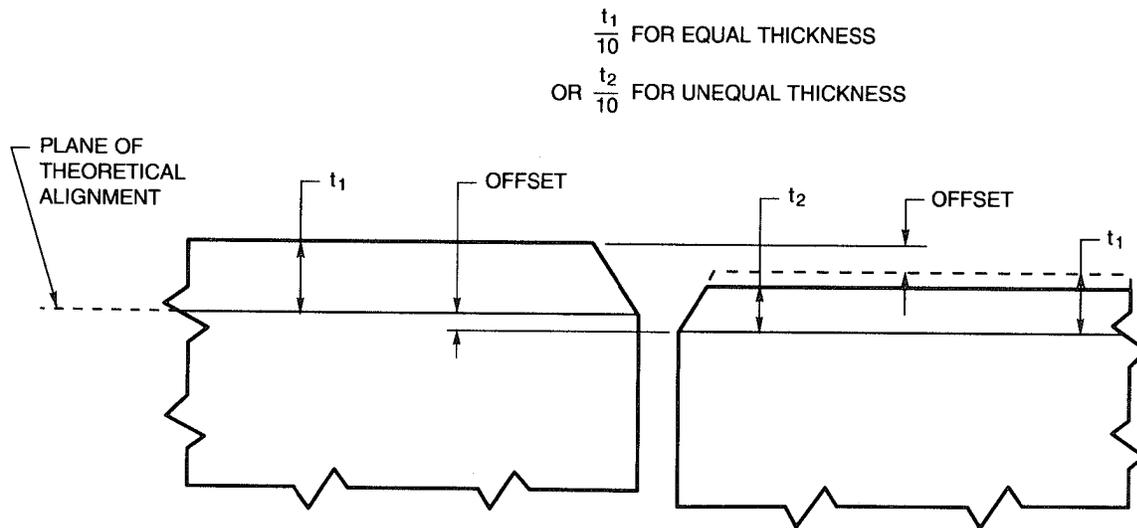
NOTE: AN OFFSET NOT EXCEEDING 10% OF THE THICKNESS OF THE THINNER PART JOINED, BUT IN NO CASE MORE THAN 1/8 in. (3 mm), MAY BE PERMITTED AS A DEPARTURE FROM THE THEORETICAL ALIGNMENT.
