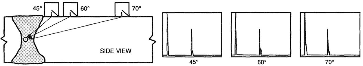
Amplitude remains unchanged (assuming equal sensitivity calibration and adjustment for attenuation), distance changes with angle (unless calibrated to be the same) as sound is moved around the discontinuity.
