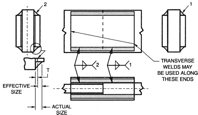
NOTE: THE EFFECTIVE AREA OF WELD 2 SHALL EQUAL THAT OF WELD 1, BUT ITS SIZE SHALL BE ITS EFFECTIVE SIZE PLUS THE THICKNESS OF THE FILLER PLATE T.
