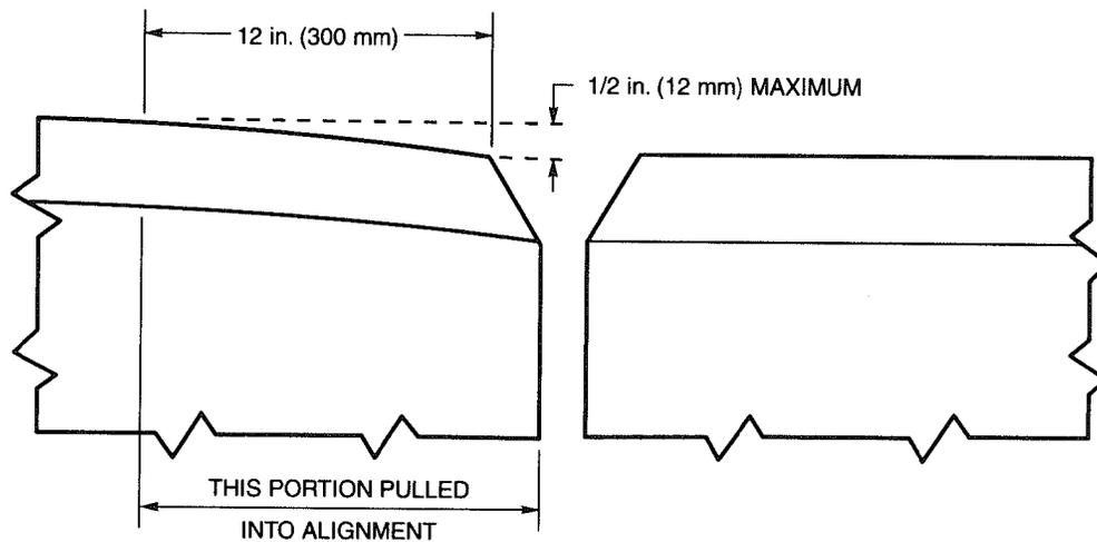
NOTE: IN CORRECTING MISALIGNMENT THAT EXCEEDS THE PERMISSIBLE ALLOWANCE, THE PARTS SHALL NOT BE DRAWN TO A SLOPE GREATER THAN 1/2 in. (12 mm) IN 12 in. (300 mm).
