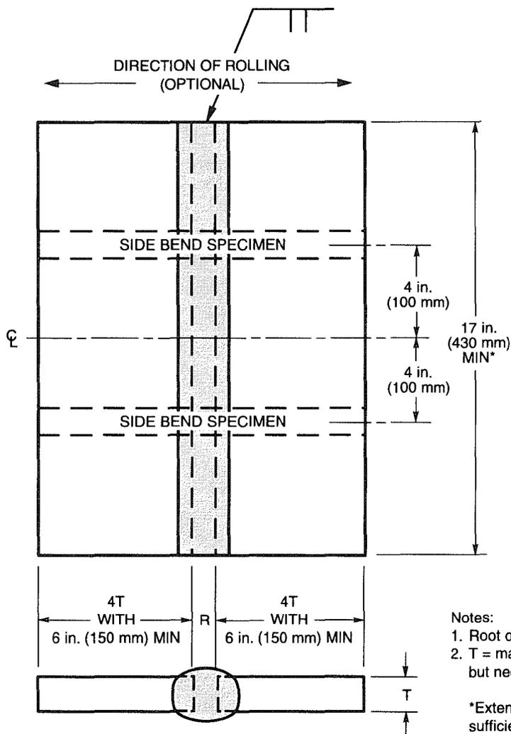
**Figure 4.35—Butt Joint for Welding Operator Qualification—
