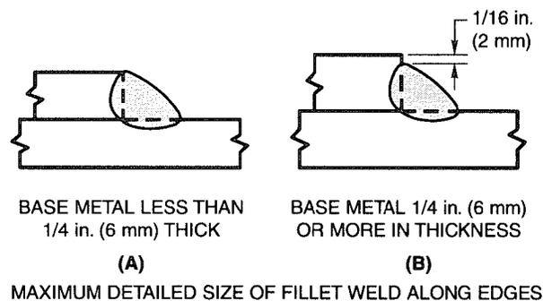
**Figure 2.1—Details for Prequalified Fillet Welds (see 2.4.5)**
