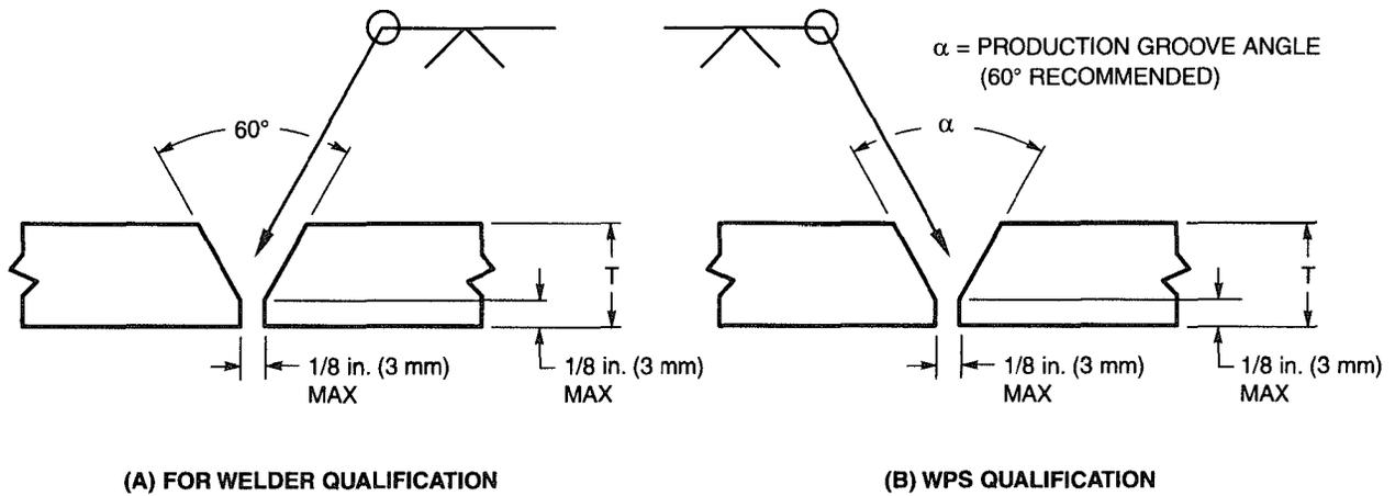
NOTE: T = QUALIFICATION PIPE OR BOX TUBE WALL THICKNESS
