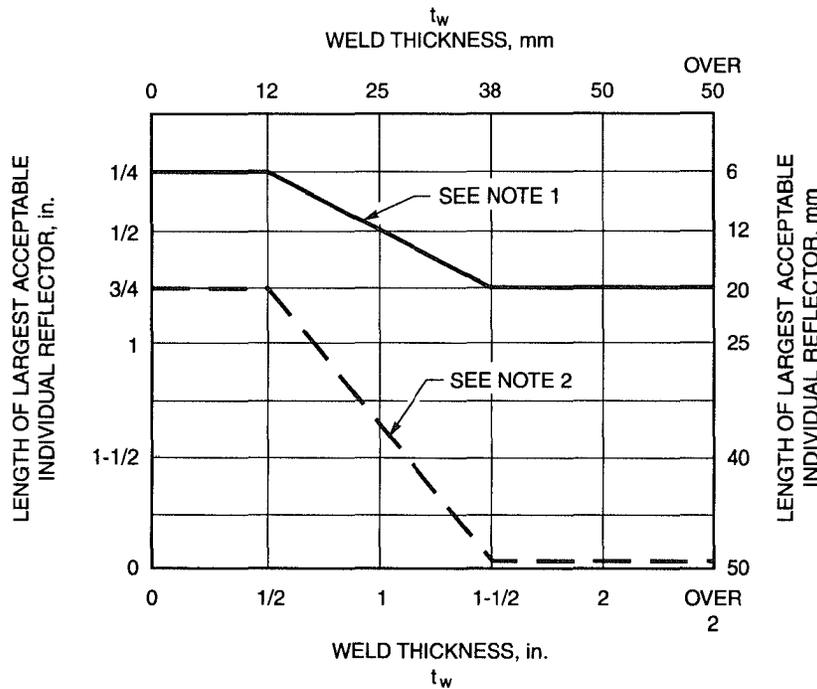
1. INTERNAL LINEAR OR PLANAR REFLECTORS ABOVE STANDARD SENSITIVITY (EXCEPT ROOT OF SINGLE WELDED T-, Y-, AND K-CONNECTIONS—SEE FIGURE 6.8).
