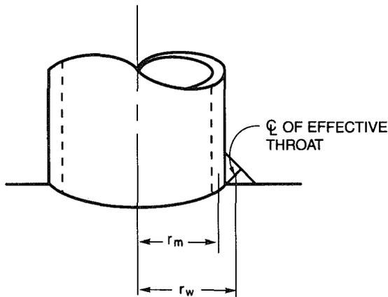
**Figure 2.16—Tubular T-, Y-, and K-Connection**
