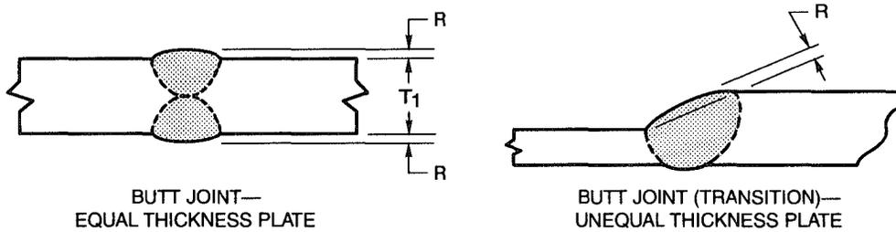
NOTE: REINFORCEMENT R SHALL NOT EXCEED 1/8 in. (3 mm). SEE 5.24.4.
