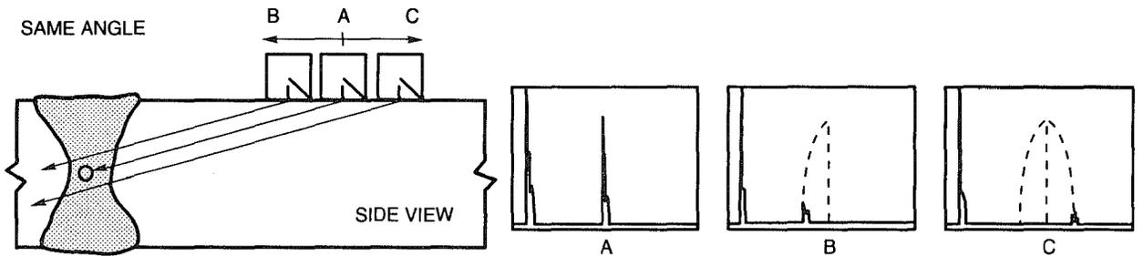
Amplitude drops rapidly showing little or no discontinuity indication with the same angle but distance changes as the search unit is moved towards and away from the discontinuity.
