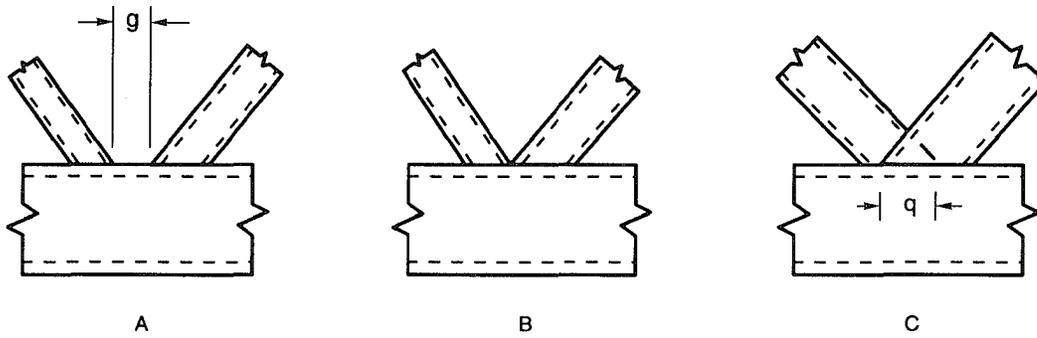
**Figure C2.23—Transition Between Gap and Overlap Connections**
