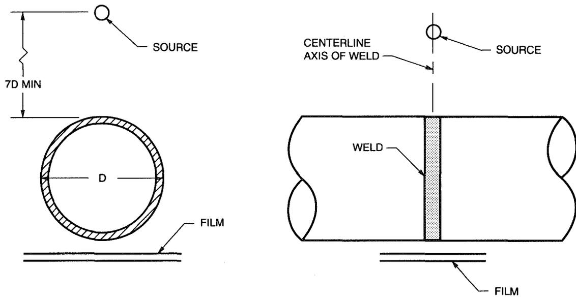
**Figure 6.19—Double-Wall Exposure—Double-Wall View, Minimum Three Exposures (see 6.18.1.3)**
