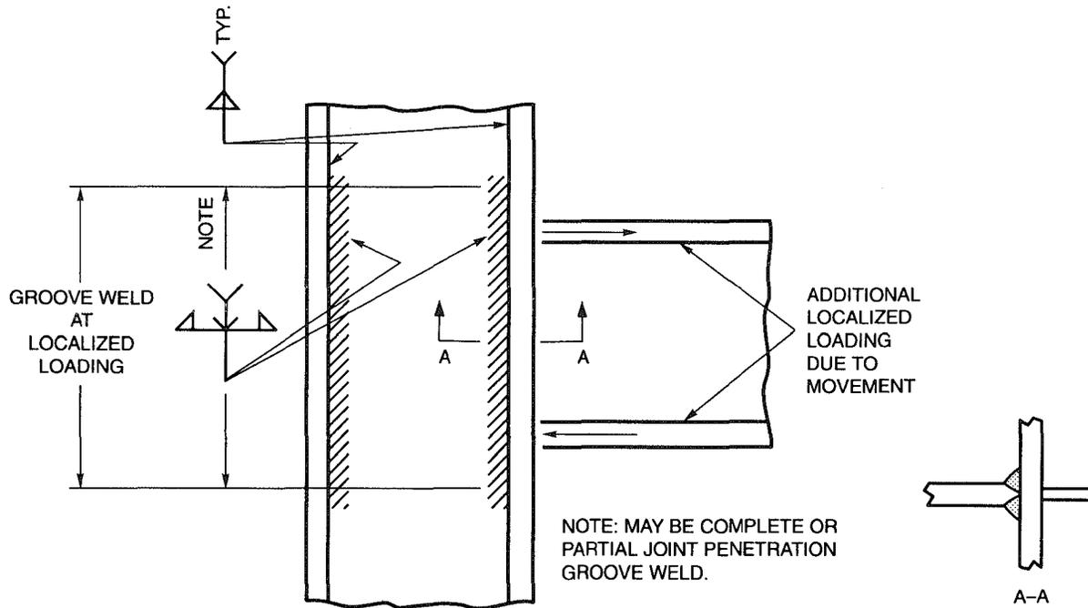
**Figure C2.24—Partial Length Groove Weld** (see 2.12)
