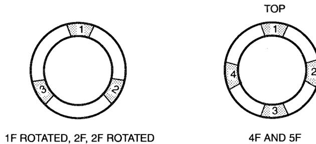
**LOCATION OF TEST SPECIMENS ON WELDED PIPE – WPS QUALIFICATION**
